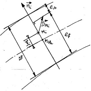
After displacement the distance es between point Mi and surface Ssupshould be negative and the distance eg between a point M; and surface Sinf should be positive, or :
