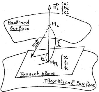
$^{\mathsf{M}}$ ; is a point of the machined surface obtained by intersection of normal n; and the machined surface. An instrument of inspection will usually measure the algebric quantity:
