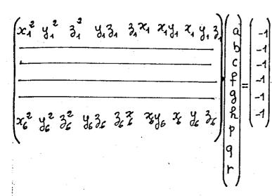
The 3 non linear equations can be solved simultaneously by the method of Newton. To find the initial value for the iterative calculation, the best method is to solve system (I) simply by adding a supplementary condition :
