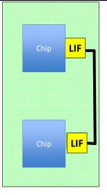
Chips are linked by *intra-device-level LIFs* to form a device.
